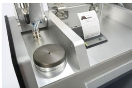
*The sample reactor within the ChocoAnalyzer instrument.*
